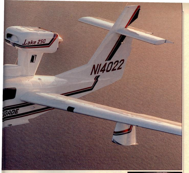
two worst cases of loading are a single occupant and full fuel (nose ballast will be required) and full cabin with partial fuel (aft ballast will probably be required to maintain CG within limits). For most operations between the extremes, ballast is not required.
